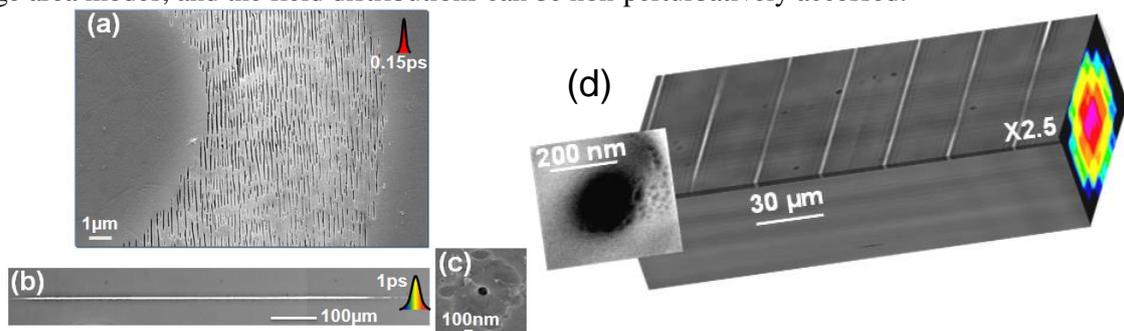
Fig1. (a-c) Examples of bulk nanostructuring in fused silica using self-organization or non-diffractive direct focusing concepts. (d) Embedded photonic device for spectrometry
